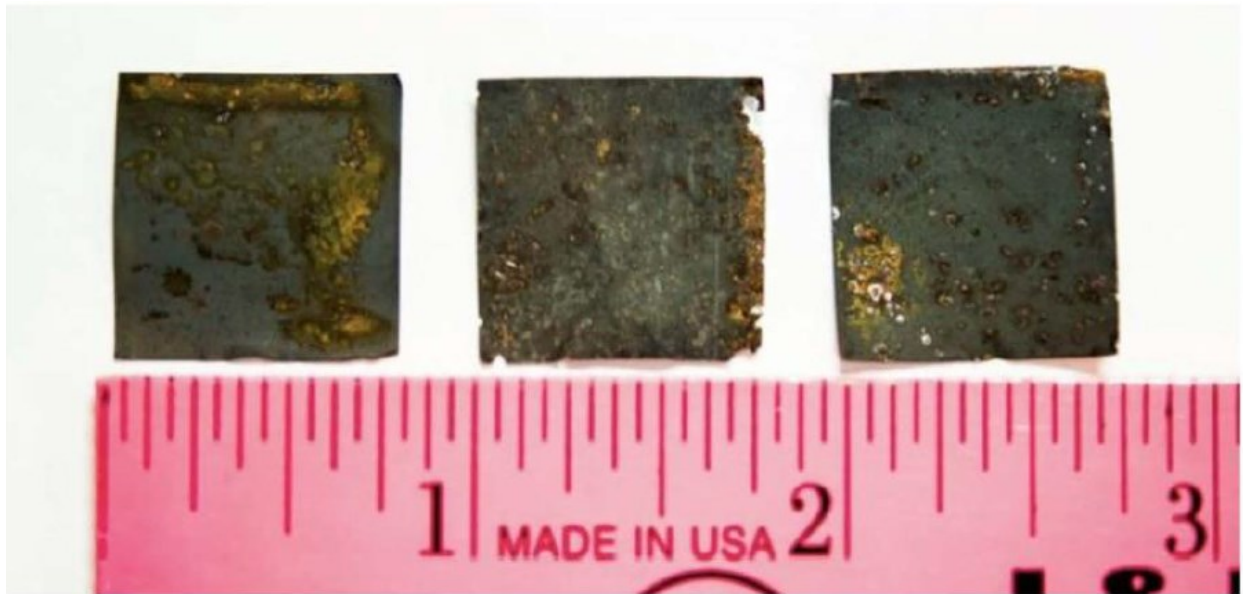
Figure 3-4 Pyrophoric Iron Foils After Deployment and Some Weathering
